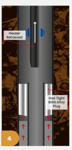
The Wel-lok™ technology consists of utilising a modified thermite chemical reaction heater to melt bismuth-based alloys downhole.
